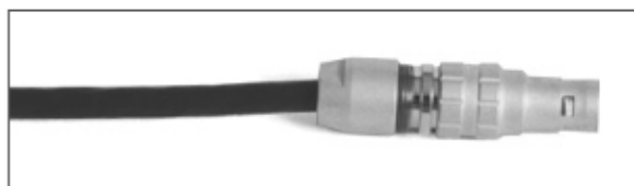
Figure 2.2d Cable connector that plugs into the computer unit has no boot.
