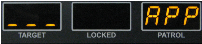
Figure 3.3.1c Stationary track Approach targets (No antenna is selected)
