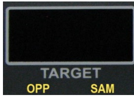
Figure 4.2.1d OPP and SAME indicator lights
